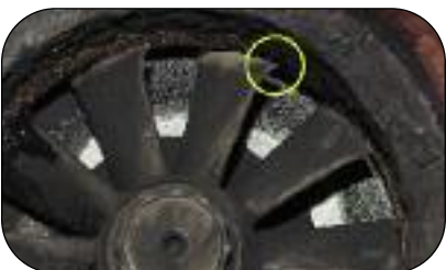
Figure 6 - Damaged Core Refund Hot wheel bent
