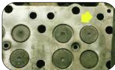
Figure 5 - Damaged Core Refund Metal stamp on combustion face
