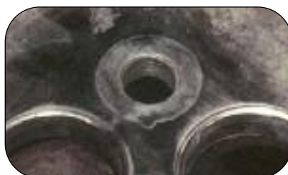
Figure 6 - Damaged Core Refund A plug which is not cast iron has been welded into this head to replace a cracked area around the bore. Perkins does not use or authorise this process
