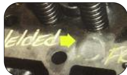
Figure 7 - Damaged Core Refund This head had a top deck crack and was repaired by welding the freeze plug hole shut. Perkins does not use or authorise this process
