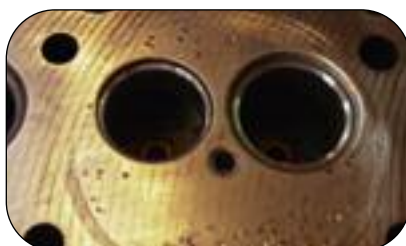
Figure 4 - Damaged Core Refund Dropped valve damage
