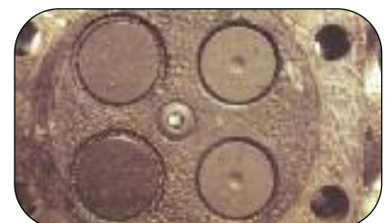
Figure 8 - Full Core Refund Pitting
