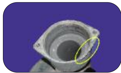
Figure 3 - Full Core Refund Damage - chipped cold housing
