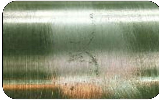
Figure 4 - No Core Refund Excessive pitting
