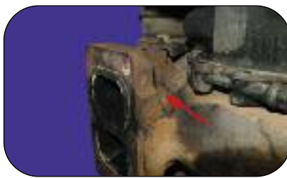
Figure 2 - Full Core Refund Operational damage - crack
