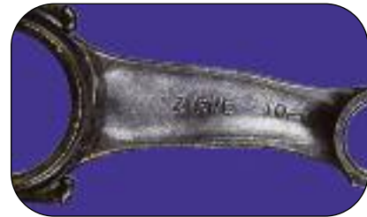
Figure 4 - No Core Refund Visibly bent and twisted
